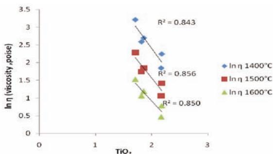
Fig.12. Effect of TiO<sub>2</sub> addition on viscosity.
