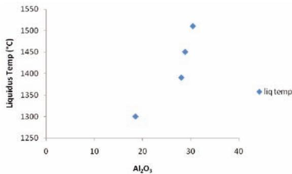
Fig.5. Effect of alumina on Liquidus temp.
