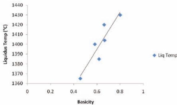
Fig.10. Effect of Basicity on Liquidus temp.
