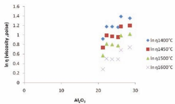
Fig.11. Effect of alumina on viscosity.
