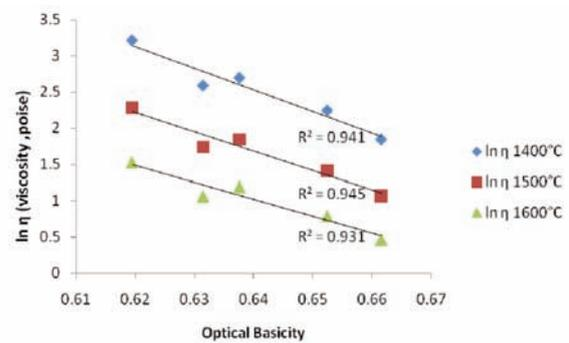
Fig.13. Effect of OB<sub>DUFFY</sub> on viscosity.
