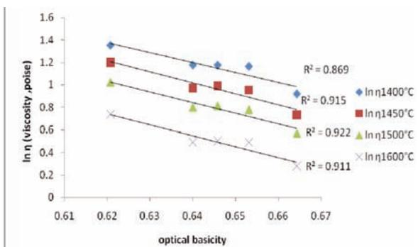
Fig.7. Effect of  $OB_{DUFFY}$  on viscosity.
